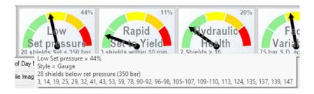
Right-click on any gauge to copy the image of all gauges to the Windows clipboard, or to copy the displayed Tooltip text for an individual gauge, or to change the gauge style between gauge/box/hybrid/hybrid with pop-up...
