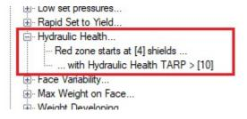
The Hydraulic Health TARP settings are also configured under these Global settings. Refer to the separate LVA info sheet "LVA Infosheet - Hydraulic Health.pdf" for a full description of the hydraulic health feature. This is what the configuration looks like...
